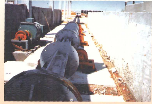
BETON DİREK KALIBI VE SANTRİFÜJ MAKİNASI ELECTRIC POLE MOULDS AND SPIN MACHINE
