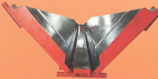
ÇATI MAKASI KALIBI ROOF BEAMS MOULD
